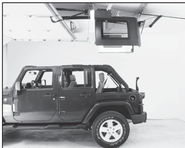
OPTION 1. Above Garage Door: Clearance to lift and store top above open garage door.
