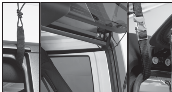
DIAGRAM 21. Run straps lengthwise from front door to rear tailgate between top and rollbar.
