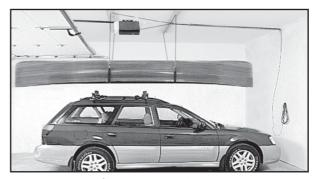
**OPTION 2.** Below Garage Door: Use if not enough clearance for Above Garage Door Storage (Option 1). Object has clearance to lift and store below open garage door.
