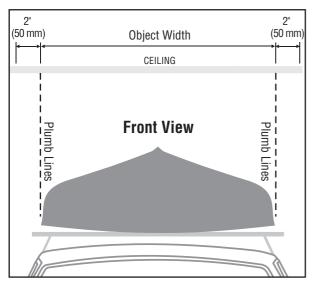
**DIAGRAM 5.** Mark object width on mounting boards.
