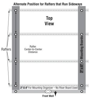
**DIAGRAM 4A.** For Alternate Position attach board for mounting organizer using  $^{5}/_{16}$ " (8 mm)  $^{3}/_{2}$ " (90 mm) lag bolts and washers (not included). See Step 3a to determine distance between mounting boards.
