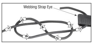
**DIAGRAM 18.** Tie a Black Drop Rope to each Webbing Strap (E) using a figure-eight knot. Pass free end of rope through the sewn Webbing Strap eye.
