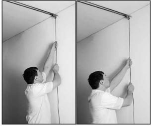
With rope pointed down the cleat will lock the rope and you can release it. Repeat until object is at desired height.
