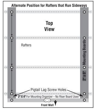
DIAGRAM 7. If rafters run sideways, drill pigtail lag screw holes on 2" x 6" as shown.
