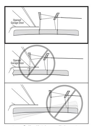
**DIAGRAM 1.** Position object above car with clearance to open garage door. If Hoister is mounted too close to garage door, there may not be clearance to open door. Mounted too far forward, object may not balance or lower onto car.
