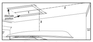
**DIAGRAM 3a.** Alternate position for rafters running sideways. Check to make sure 6' (1.83 m) boards are long enough.
