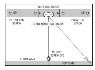
**DIAGRAM 12.** If distance to front wall is less than distance needed to lift object, move the Welded Screw Eye (A) along the front wall until distance 2 is equal to distance 3 (see Diagram 11).
