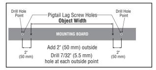
**DIAGRAM 6.** Add 2" (50 mm) outside each mark. Drill a <sup>7</sup>/32" (5.5 mm) hole at each drill point on mounting boards
